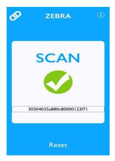
5. Once the EPC barcode is also scanned the application will navigate to Write to tag screen. Here it allows to write the generated tag data into the corresponding tag.
